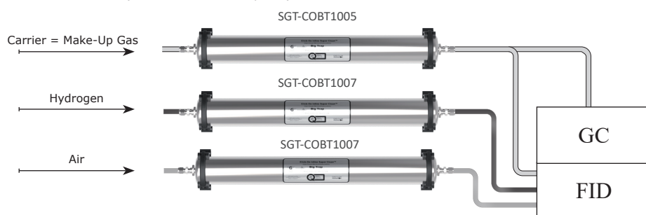
GC/FID Solution 1 (Carrier Gas = Make-Up Gas)
